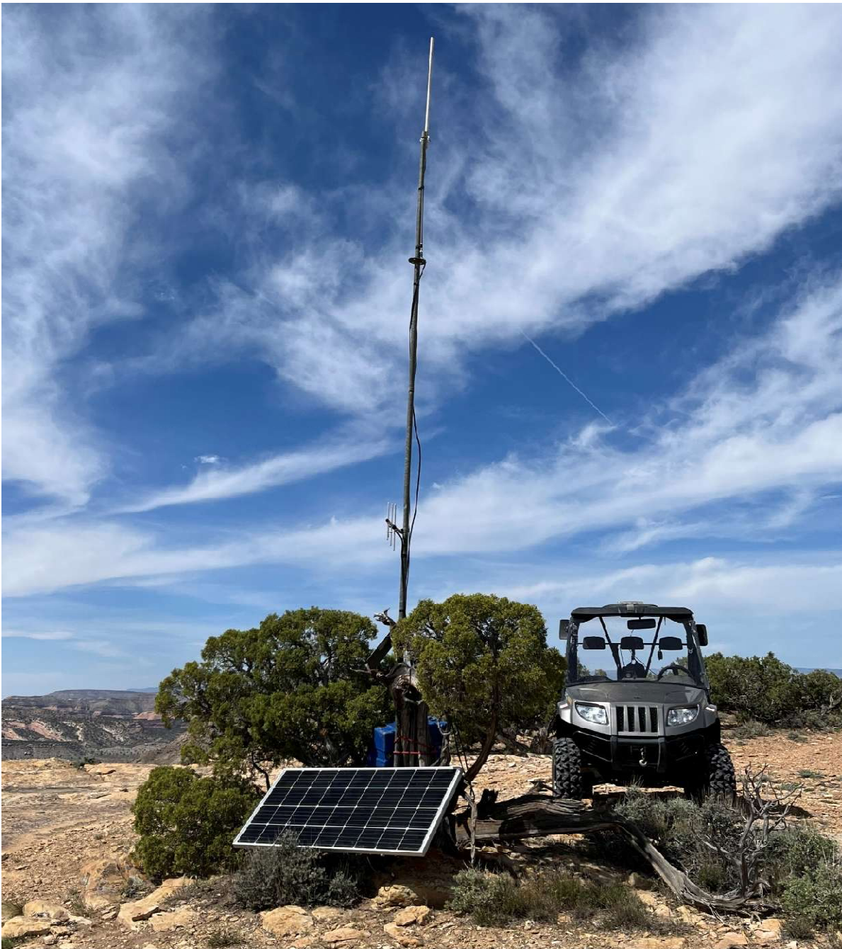
Keri's second portable repeater site, including Meshtastic node.
