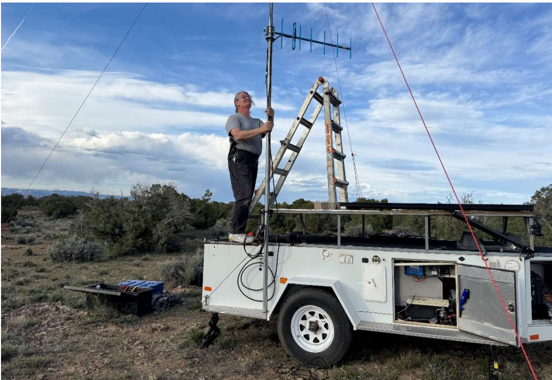
Keri N2KNK setting up the portable comm trailer, containing portable repeater, APRS digipeter and Meshtastic node, with a full solar and battery system.
